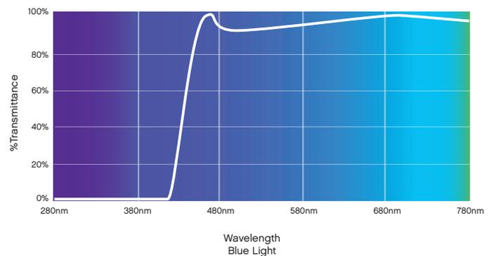
**Figure 8:** One manufacturer's claim of a "clear" lens, results in a dip in transmittance below 90% from 490-540 nm. Will this result in diminished visual performance?
