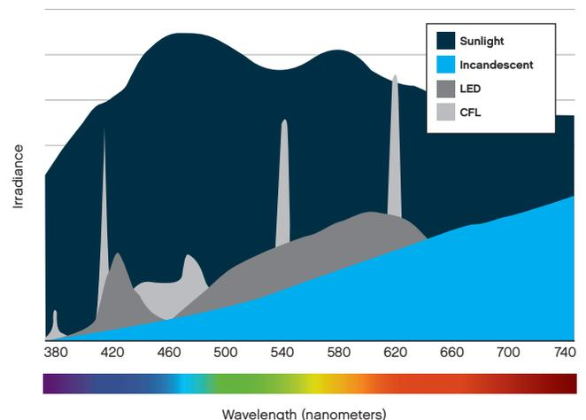
**Figure 2:** Visible spectra of common light sources. Note that sunlight is the strongest source of blue light we are exposed to, while incandescent light bulbs emit the least blue light of electric light sources.
