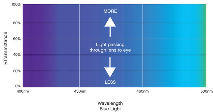
**Figure 6:** In defining how a spectral transmittance graph denotes the properties of a given spectacle lens, note that a higher transmittance value along the x-axis indicates more light is passing through the lens.
