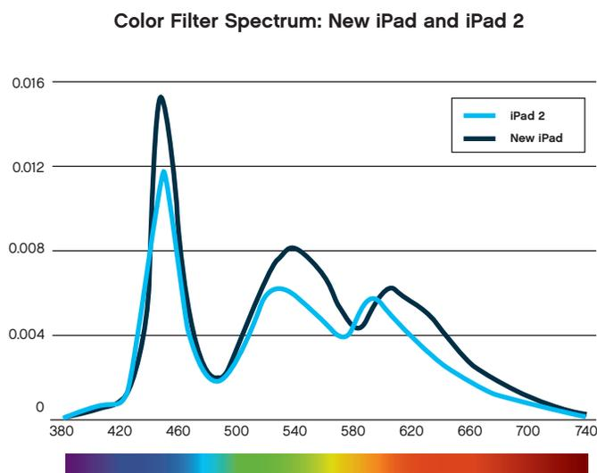
**Figure 3:** iPad 2 released March 2, 2011 vs. the New iPad with Retina Display released March 7, 2012. Note the increase in the spectral emission in the blue peak at 450 nm. Also note that there is almost twice as much blue light emitted as green light, and over four times as much blue light emitted as there is red light.<sup>5</sup>
