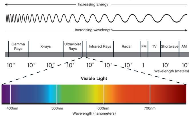
**Figure 1:** The electromagnetic spectrum. Note that as energy increases, the wavelengths get shorter. Blue light ranges from 400-500 nm, having the shortest wavelengths of visible light, thus having the highest energy.
